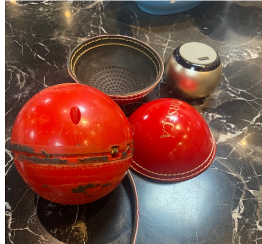
Retrofitting a Bluetooth receiver and sound driver to create the UpBeat Speaker using a cricket ball
