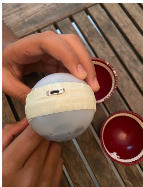
Securely taping the two halves of the PVC Ball together
